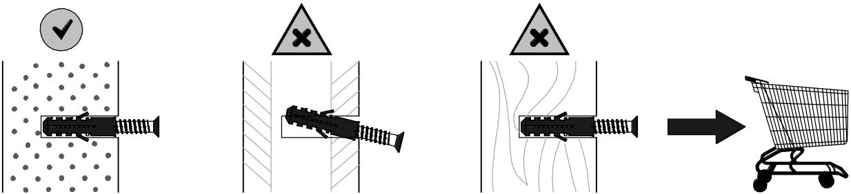
**- EN -** Before suspending or fixing furniture to the wall (in order to prevent falling over), check the type and strength of the wall. Select wall plugs and screws appropriate for the given type of the wall. In the case of doubts, contact a specialist. The installation must be performed by a competent person. **WARNING!!! If the rawlplugs with screws are attached to the product, then they are intended only for walls made of solid and homogeneous materials.**
